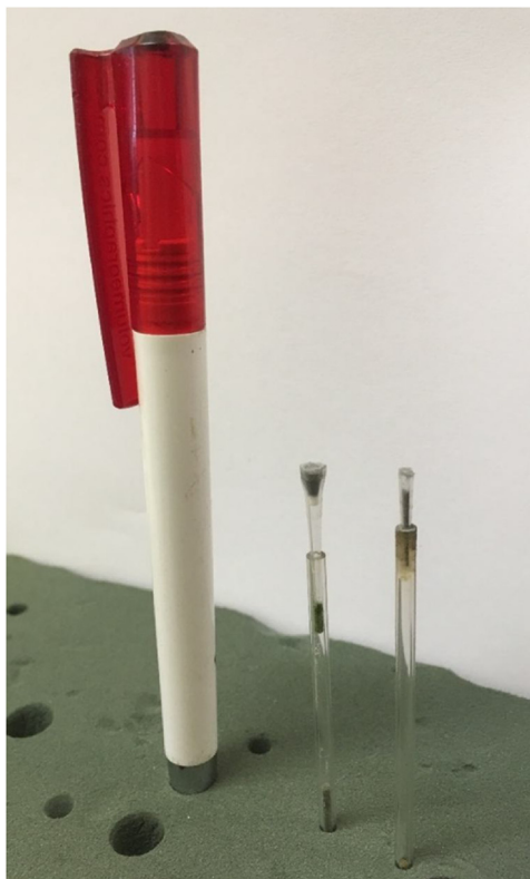
Fig. 1. Sample mounting – the pen is for scale indication, the powder is loaded in the cup or tube as shown – sample on left is for 1.5 \mu\text{m} scan, sample on right is for smaller powders for 0.7 \mu\text{m} scan.
