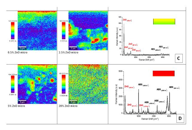
**Figure 8.** Raman mapping and spectra of micro-ZnO-ABS printed composite materials. (**C**) Example of a Raman spectrum corresponding to yellow-green color regions in the maps; (**D**) example of Raman spectrum corresponding to red color regions in the maps.
