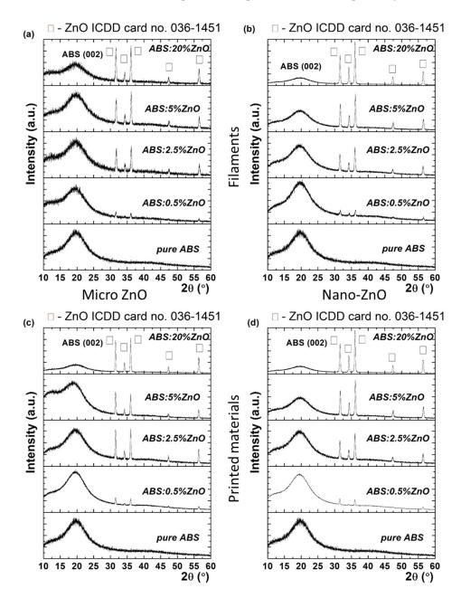
**Figure 3.** XRD patterns of micro- (**a**) and nano-ZnO-ABS (**b**) filaments, micro- (**c**) and nano-ZnO-ABS (**d**) printed materials, as well as for pure ABS.
