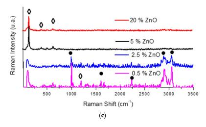
**Figure 6.** (a) Raman spectra of 20% micro- and nano-ZnO-ABS printed composite materials; (b) Peak analysis of Raman spectrum for 20% micro-ZnO-ABS; and (c) Raman spectrum for micro-ZnO-ABS composites as a function of ZnO concentration.
