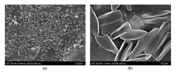
**Figure 13.** Higher magnification SEM images of (**a**) *Chlorella* biofilm on the 5% nano-ZnO-ABS and (**b**) *Navicula* biofilms on the 5% micro-ZnO-ABS, 3D printed composites.
