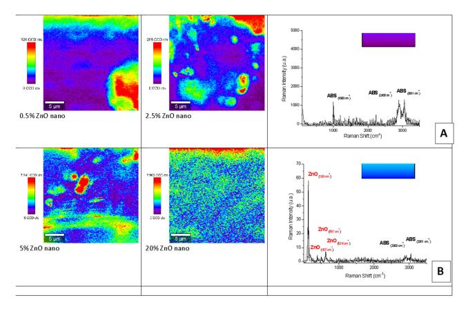
**Figure 7.** Raman mapping and spectra of nano-ZnO-ABS printed composite materials. (**A**) Example of Raman spectrum corresponding to mauve-blue dark color regions in the maps; (**B**) example of a Raman spectrum corresponding to blue color regions in the maps.
