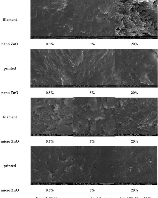
**Figure 5.** SEM images presenting examples of the structures of the 0.5%, 5% and 20% nano- and micro-ZnO-ABS filaments and printed composite materials. Magnification  $\times$  20,000. Scale is 4  $\mu$ m for all images.
