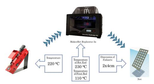
Figure 1. The used printing system and the growth conditions.
