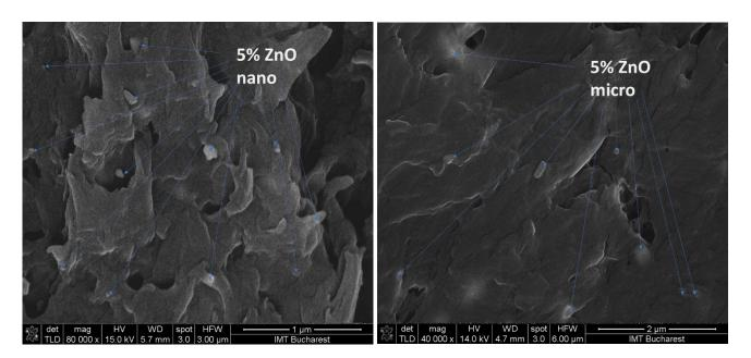
Figure 4. High magnification FESEM for the 5% ZnO nano- and micro- samples; 5% nano ZnO-ABS  $\times$  80,000; 5% micro ZnO-ABS  $\times$  40,000.
