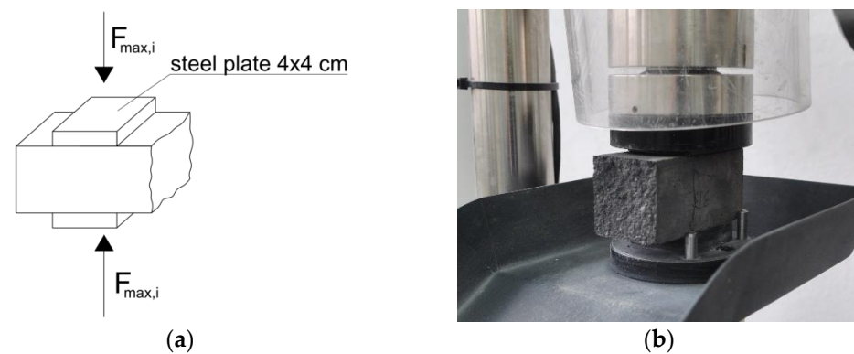
Figure 2. Determination of compression strength: (a) static scheme, loading, and geometry of tested specimens; (b) the view of the specimen ready to test.
