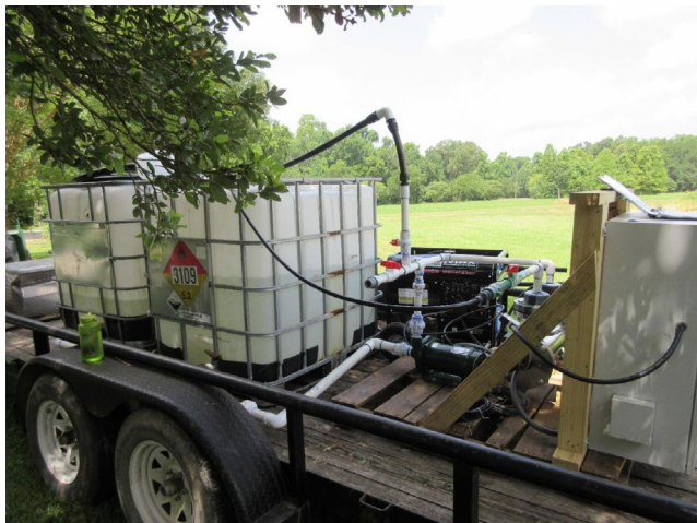
FIGURE 1 UV-C treatment system (PMD 150C1/4, Aquionics, Slough, UK) for irrigation water. LSU AgCenter Botanical Garden, Baton Rouge, Louisiana
