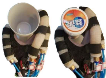
FIGURE 17. Grasping test of rehabilitation glove without the glove wearing on the hand.
