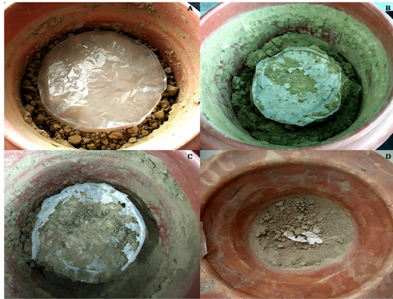
Fig 7. Soil burial method for the degradation of PHB film as compared with (A) control after treatment with the Aeromonas caviae Kuk1-(34) sp. for (B) 15 days (C) 30 days and (D) 45 days.
