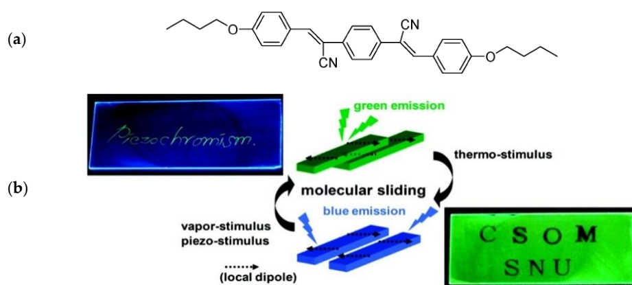
Figure 4. (a) Chemical structure of the cyano-substituted distyrylbenzene derivative; (b) Illustration of two different modes of slip-stacking in dye molecular sheets, dictated by different ways of the antiparallel/head-to-tail coupling of local dipoles and photos of the luminescence writing/erasing cycle of the dye/PMMA blend film. Reprinted with permission from [94]. Copyright (2010) American Chemical Society.
