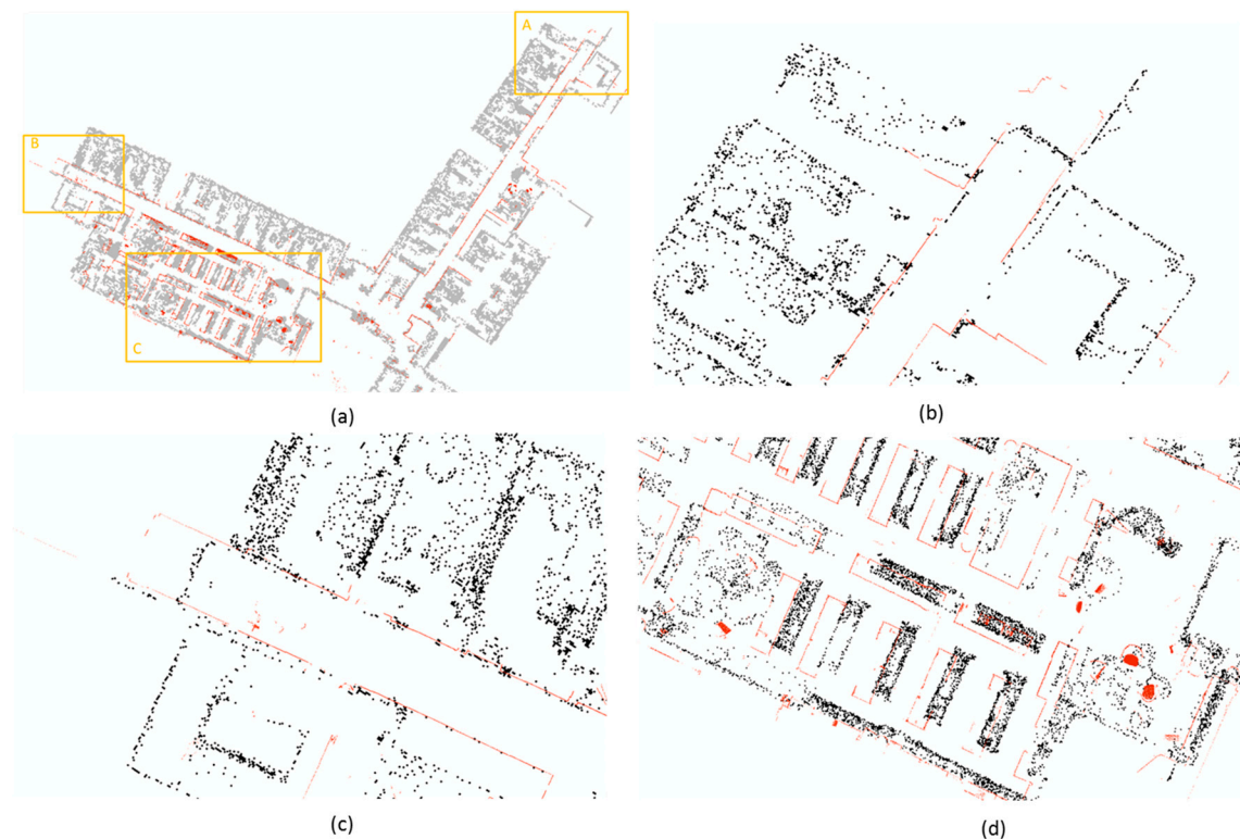
Figure 7. Mapping results comparison between T1 with TLS reference, where TLS reference is illustrated in red color against the black point cloud collected by Matterport (a) an overview comparison, (b) details at the end of east wing, (c) details at the end of south wing, (d) details of the open library in south wing.
