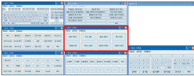
Fig. 5. The Clicky2.0 automatically scans each item (alphabets, commonly used words and sentences) according to the order and time interval previously set up. When a patient blinks his eye at the intended moment, a Self-Calibrating Auditory Tone Infrared switch is activated.
