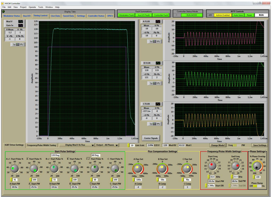
Fig. 2. Screenshot of the RFTF controller screen showing the tuning/setting knobs and live waveform diagrams.
