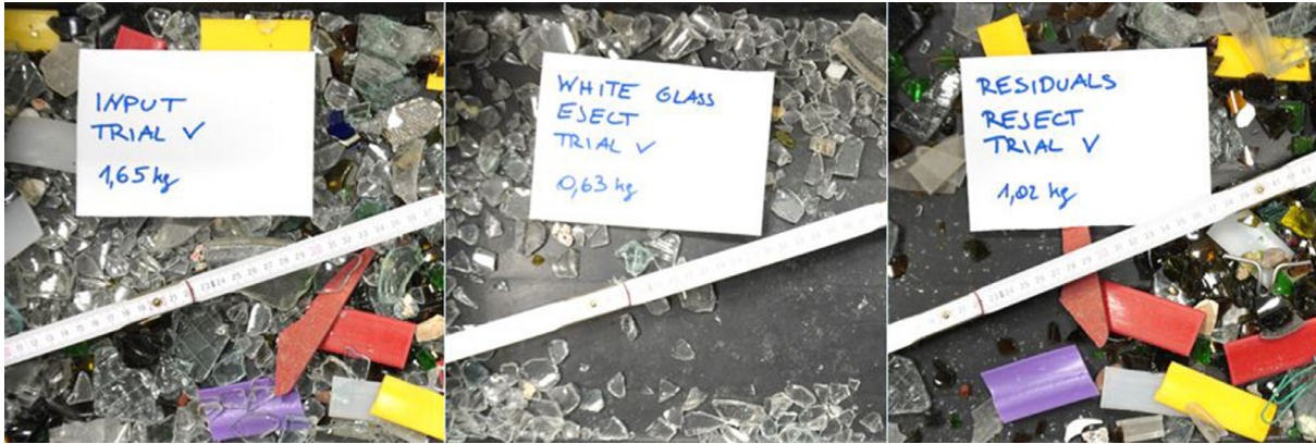
Fig. 17. Feed material (left), separated white glass – Eject (centre) and residuals – Reject (right) (Trial 5 of Table 12) (authors depiction).
