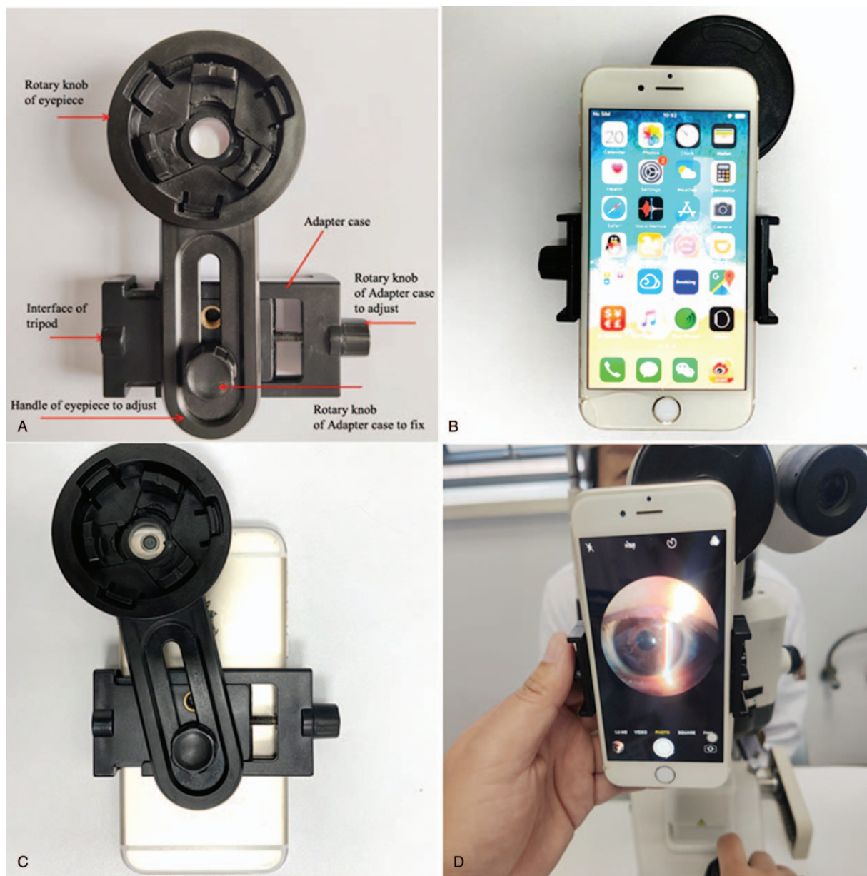
Figure 2. (A) Structure of adapter; (B) A universal eyepiece adapter and a smartphone; (C) A smartphone with an interface eyepiece adapter mounted on a slit lamp to capture anterior segment imaging.
