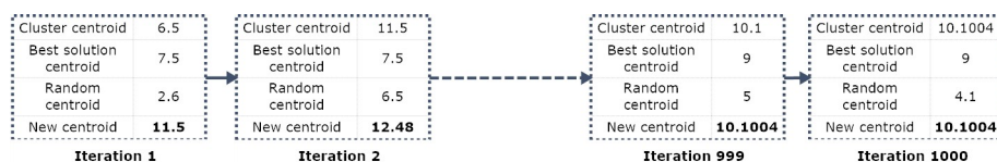
Fig 7. Example of the adaptive DE strategy performed on a cluster centroid of value 6.5 throughout 1000 iterations.
