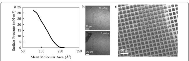
Fig. 4 Molecular design and synthesis of 2DP a surface pressure-mean molecular area isotherm, **b** Brewster angle microscopy images of the water surface after diffusion of 1 at surface pressure of 5 mN·m<sup>-1</sup> and 20 mN·m<sup>-1</sup>, and **c** SEM image of UV-irradiated monolayer film on a TEM grid
