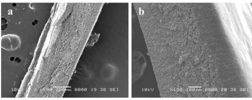
**Fig. 6** Measuring thickness using SEM image of cross sections Thickness of each cell-plastic is evaluated using SEM image of cross section. **a** Cell-plastic (Gly) and **b** cell-plastic (Gly-BSA) under magnifications of × 90 and × 130, respectively
