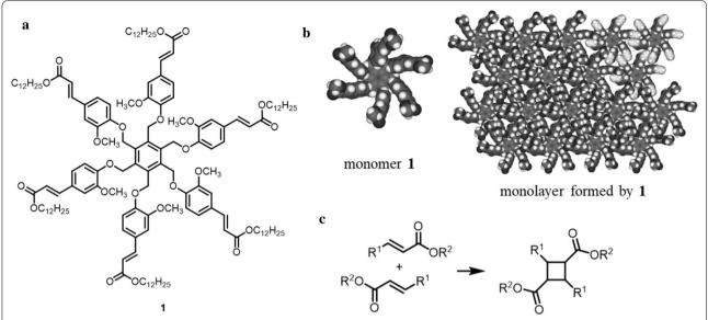
**Fig. 2** Chemical structure and molecular models **a** Chemical structure of monomer 1, **b** molecular models of 1 (left) and monolayer formed by 1 (right), and **c** chemical reaction of photocycloaddition of cinnamate derivative. In (**b**), C<sub>12</sub> alkyl chains and some of the cinnamate units at an upper right part of the model of the monolayer are omitted for clarity reason
