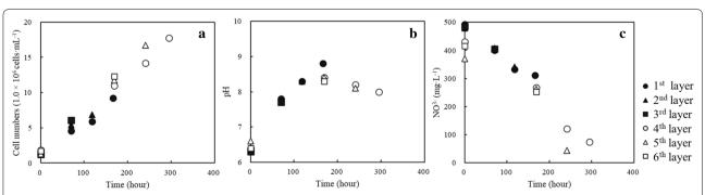
**Fig. 3** Broth condition of *C. reinhardtii* in each culturing system Time-course profiles of **a** cell number, **b** pH, and **c** nitrate concentration are shown as closed circle (1st layer), closed triangle (2nd layer), closed square (3rd layer), opened circle (4th layer), opened triangle (5th layer) and opened square (6th layer). Harvested points were 70 h (1st layer), 118 h (2nd layer), 166 h (3rd layer), 169 h (4th layer), 241 h (5th layer) and 295 h (6th layer), respectively
