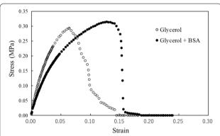
**Fig. 5** Young's modulus and tensile strength Stress–Strain curves of cell-plastic (Gly) (white circle) and cell-plastic (Gly-BSA) (Black circle). Their tensile strengths (maximum stresses) and Young's modulus (slope of the initial growth) are detected to be 0.29 MPa and 9.0 MPa (white circle), and 0.32 MPa and 6.2 MPa (Black circle), respectively
