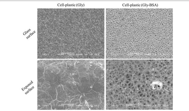
**Fig. 7** SEM images of surfaces of cell-plastic (Gly) and cell-plastic (Gly-BSA) SEM images of surfaces of cell-plastic (Gly) and cell-plastic (Gly-BSA) on left and right column, respectively. Additionally, SEM images of different surfaces are shown (upper row: glass surface; lower row: exposed surface). All magnifications were × 500
