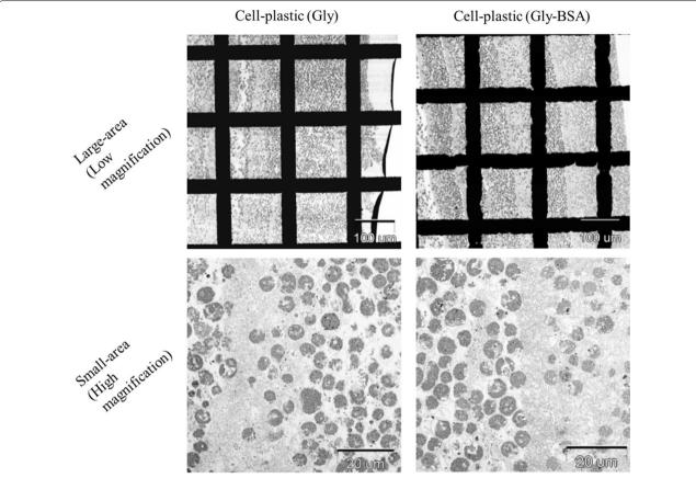
**Fig. 8** TEM images of cross sections of cell-plastic (Gly) and cell-plastic (Gly-BSA) TEM images of cell-plastic (Gly) and cell-plastic (Gly-BSA) on left and right column, respectively. Additionally, TEM images under different magnifications are shown (upper row: large area (magnification of  $\times$  126); lower row: small area (magnification of  $\times$  842))
