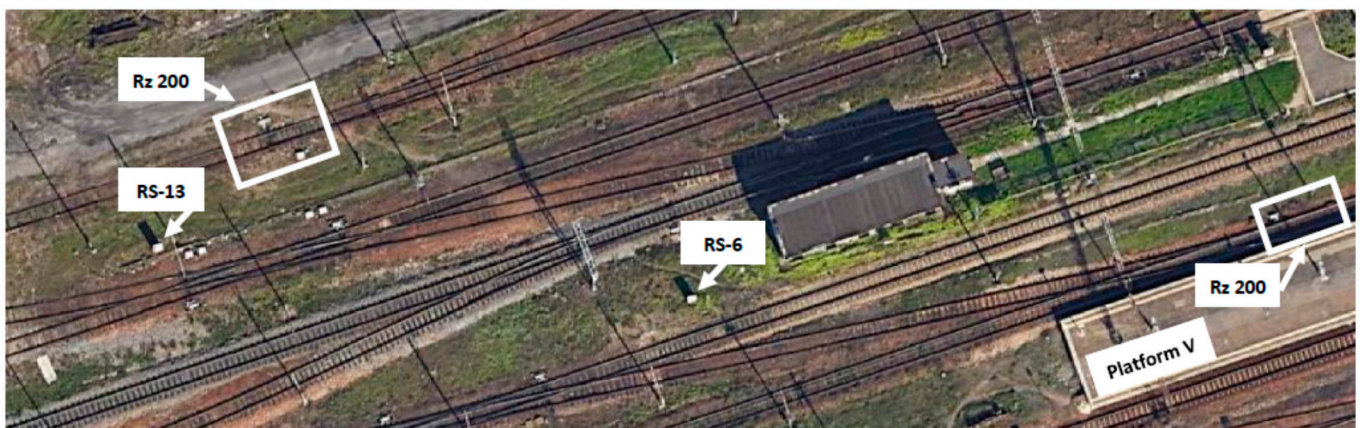
Figure 7. Satellite photo of a part of the track layout of the Warszawa Zachodnia station with marked turnouts and the apparatus and supply cabinets assigned to them (source: authors).
