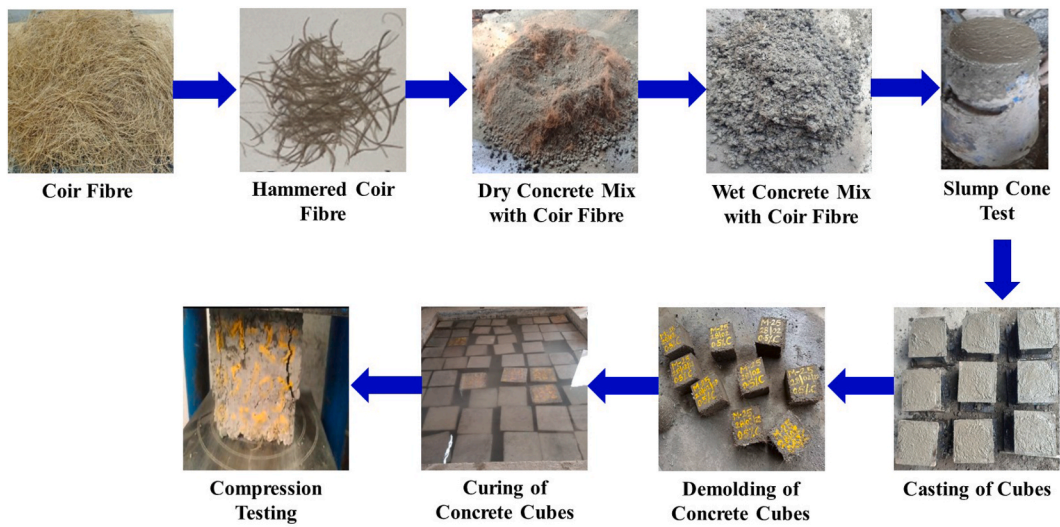
Fig. 3. Process followed for preparation of coir fibre reinforced concrete cubes.
