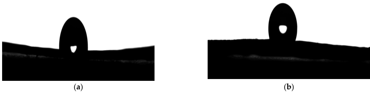
Figure 2. Contact angles of unmodified and modified straw fiber films: (a) unmodified samples; (b) modified samples.
