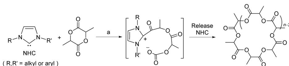
**Figure 14.** Synthesis of cyclic polymers by zwitterionic ring opening. Reagents and conditions: a) THF, 25 °C, 10 min, 81–97%. Reproduced with permission from Ref. [95]. Copyright 2011, John Wiley and Sons.
