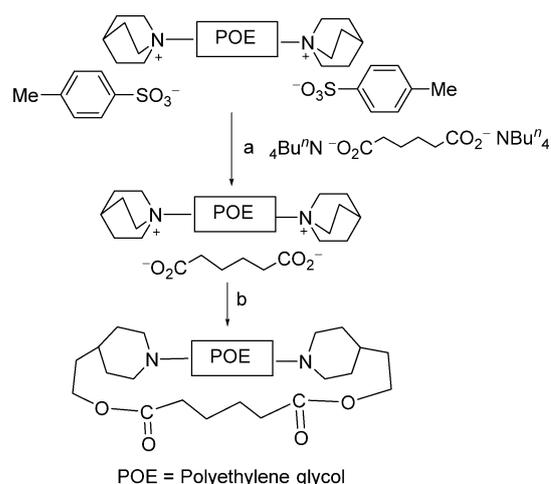
**Figure 2.** Cyclization via backbiting and covalent fixation. Reagents and conditions: a) acetone, 0°C, 0.5 h, 99%; b) toluene, reflux, 30 h, 100%. Reproduced with permission from Ref. [39]. Copyright 2002, American Chemical Society.
