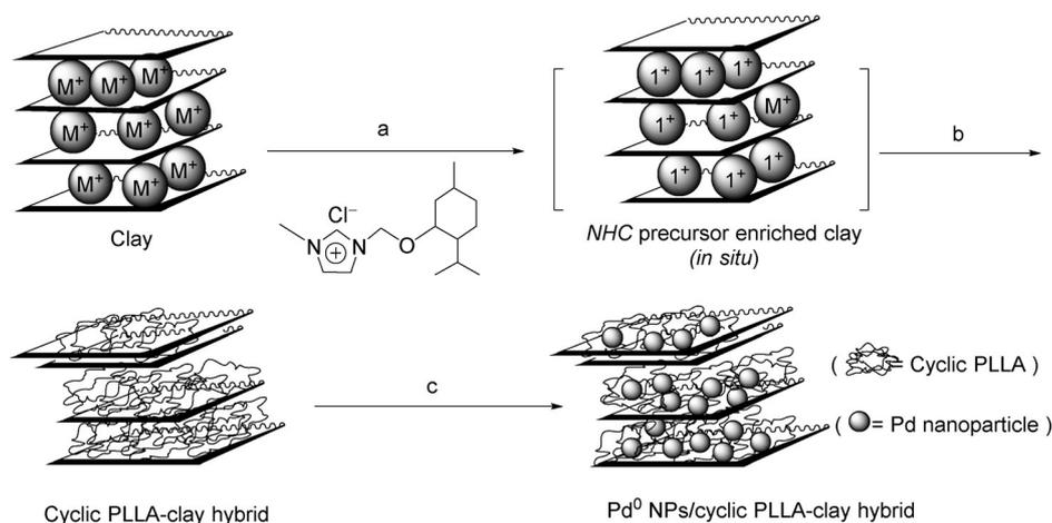
**Figure 18.** Synthesis of Pd NPs/cyclic PLLA/clay hybrids. *Reagents and conditions:* a) THF, 60 °C, 4 h; b) *n*-BuLi, L-LA, 0 °C–rt, 1 h, 80%; c) Na<sub>2</sub>PdCl<sub>4</sub>, H<sub>2</sub>O, NaBH<sub>4</sub>, dimethylformamide, –10 °C, 2 h, 95–98%. Reproduced with permission from Ref. [97]. Copyright 2013, John Wiley and Sons.
