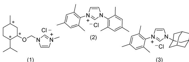
**Figure 15.** Structures of *N*-heterocyclic-carbene (NHC)-based catalyst precursors. Reproduced with permission from Ref. [96]. Copyright 2012, John Wiley and Sons.
