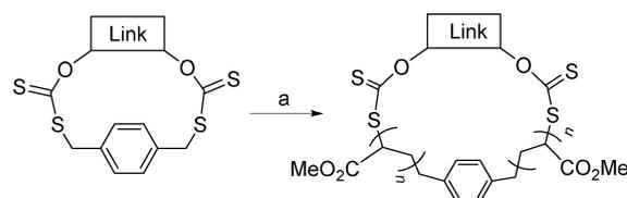
**Figure 13.** Reversible chain transfer reaction initiated by  $^{60}\text{Co}$ - $\gamma$ -irradiation. *Reagents and conditions:* a) methyl acrylate (MA),  $^{60}\text{Co}$   $\gamma$ -irradiation, THF, –30 °C, 4 h, 52%. Reproduced with permission from Ref. [92]. Copyright 2003, American Chemical Society.
