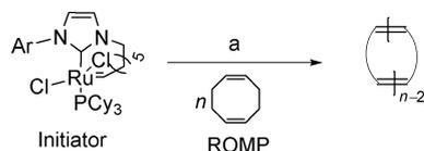
**Figure 11.** Synthesis of cyclic polymers by ring-opening metathesis reaction (ROMP). *Reagents and conditions:* a) 1,5-cyclooctadiene,  $\text{CH}_2\text{Cl}_2$ , 45 °C, 12 h, 83–95%. Reproduced with permission from Ref. [79]. Copyright 2003, American Chemical Society.
