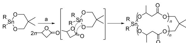
**Figure 12.** Synthesis of cyclic polymers by organotin initiator. *Reagents and conditions:* a)  $\text{CH}_2\text{Cl}_2$ , 75 °C, 6 d, 95%. Reproduced with permission from Ref. [85]. Copyright 1995, American Chemical Society.
