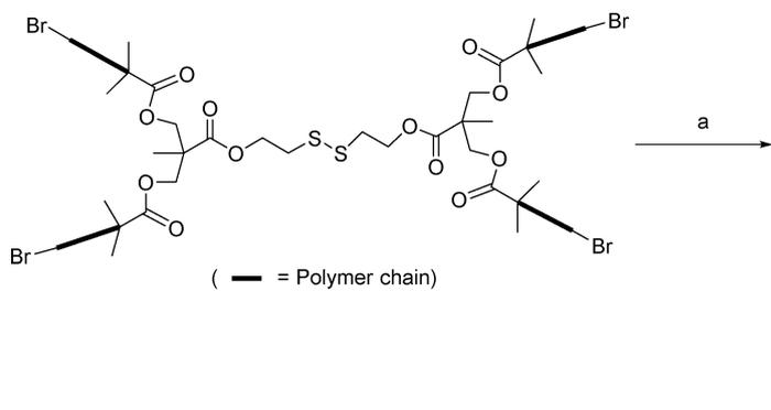
**Figure 9.** Formation of cyclic topology isomers via intramolecular ATRC. *Reagents and conditions:* CuBr/Cu/Me<sub>6</sub>Tren, THF, rt, 28 h. Reproduced with permission from Ref. [65]. Copyright 2014, American Chemical Society.
