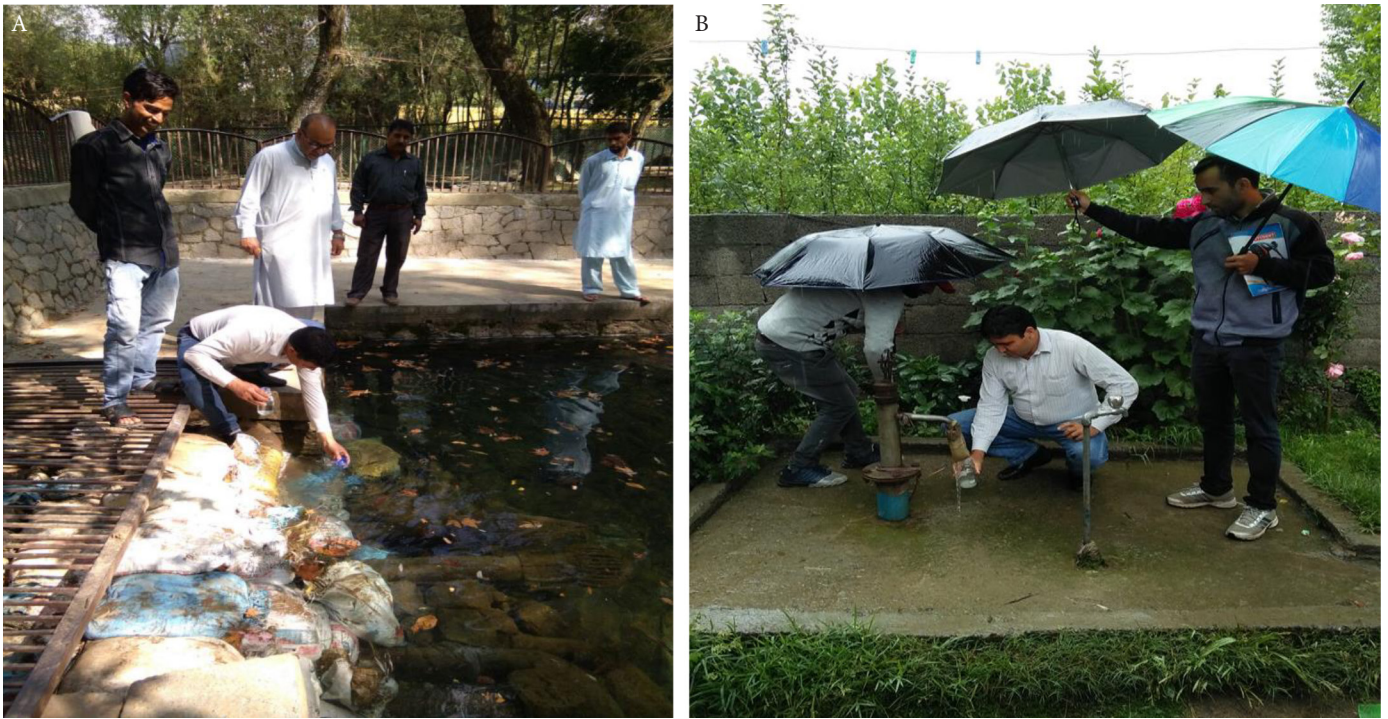
Figure 1 | (A) Water sample collection at open source. (B) Water sample collection at a bore well (hand pump)
