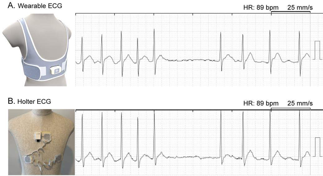
**Figure 2. Simultaneous tracing from wearable ECG (A) and Holter ECG (B).** Electrodes were positioned to compose a bipolar lead CC5 in both ECG devices. ECG, electrocardiogram; HR, heart rate.
