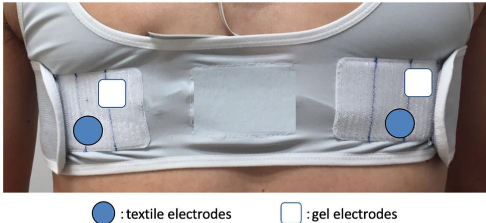
**Figure 1. Simultaneous positioning of textile and gel electrodes.** Bipolar electrodes for CC5 lead were positioned to avoid interference between textile and gel electrodes.
