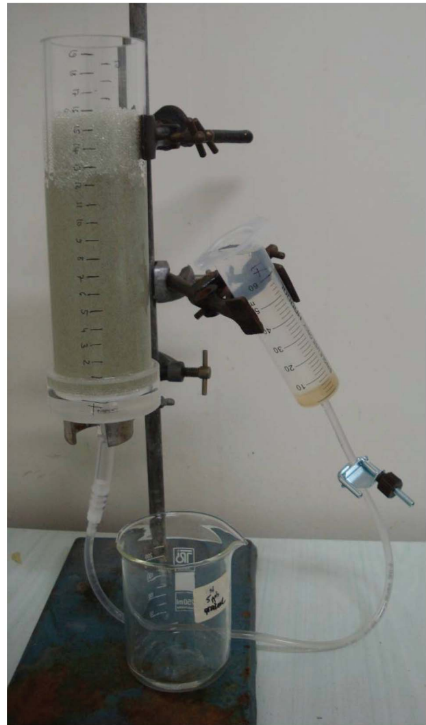
Figure 1. Experimental setup investigating the impact of drawdown on stygofauna. Column filled with glass beads and with water table lowered to 8 cm; note the unsaturated zone in the top 4 cm and the apparently saturated capillary fringe from 8–4 cm; Photo C Stumpp.
