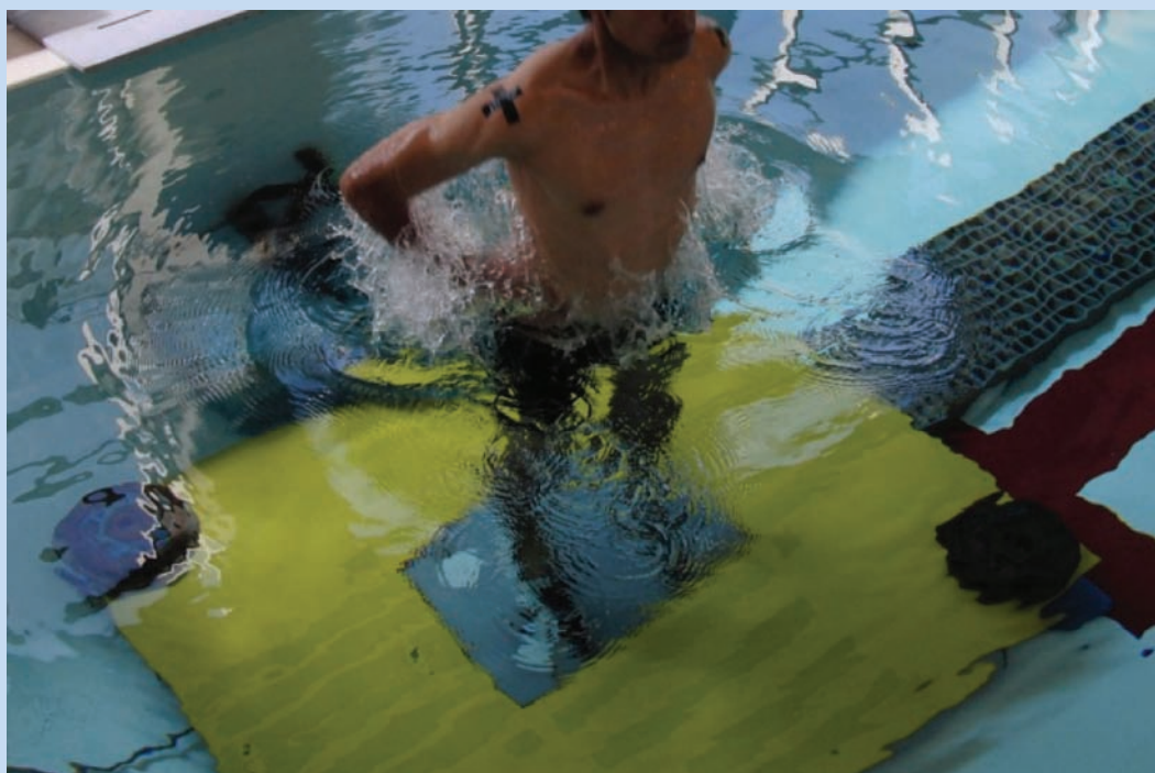
Figure 1. Force plate embedded in a platform on the floor of the swimming pool.
