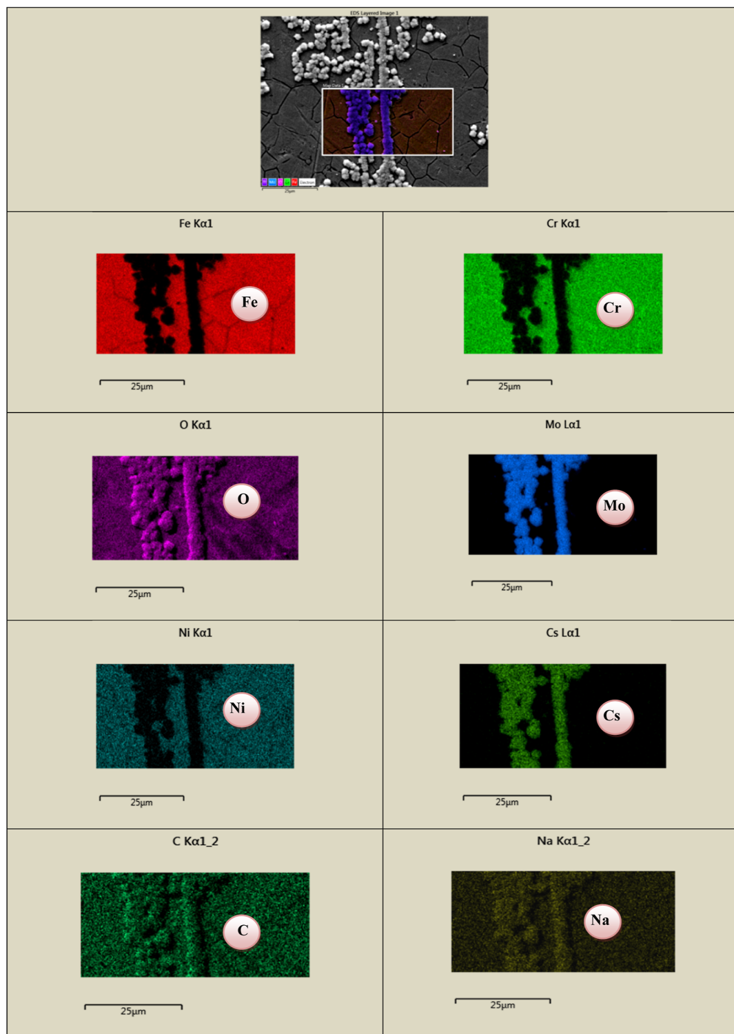
Figure 3. X-ray elemental mapping of the passivated layer with a crystallite on the metal surface.
