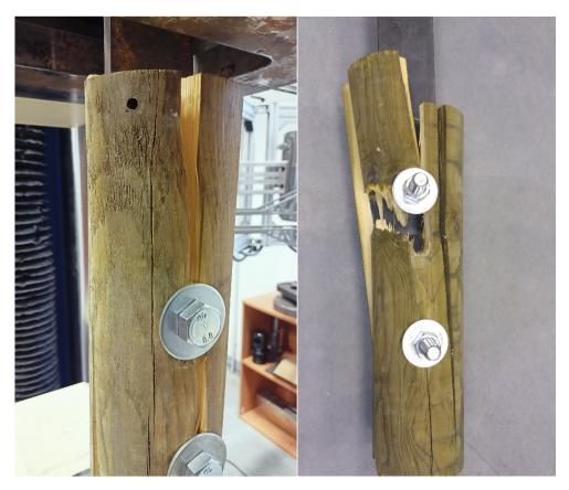
Figure 20. Specimens of round timber connections after failure.
