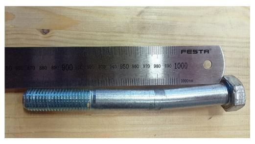
Figure 24. Deformed bolt after the experimental testing.
