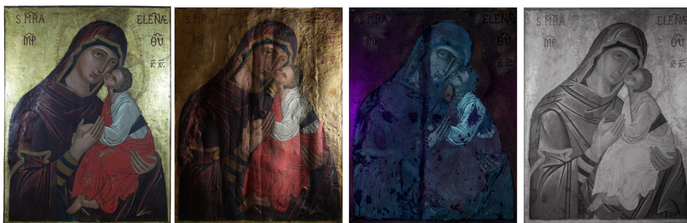
Figure 1. The Icon Madonna dell'Elemosina (Biancavilla (CT), Italy). From (left) to (right): photo in diffused vis light; vis grazing light; UV fluorescence; IR reflectography.
