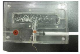
In order to stimulate the excitatory nerve to the opener muscle the preparation is now moved to a recording chamber designed with a plastic suction electrode. Having the stimulating electrode built into the chamber avoids having to use a micromanipulator to place a stimulating electrode. Pin the preparation down in the recording dish and place the branch of the nerve that contains the excitatory nerve in the suction electrode.
