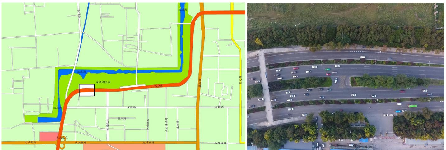
**Fig 4. A median opening at northwest corner 2nd loop road in Xi'an.** Coordinates:108.903898,34.301482. a:The U-turn median opening location schematic. b: The present median opening graphic took by a drone at height of 150m.
