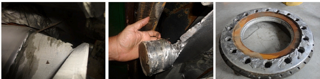
Fig. 5. Wear on the Francis turbine at the Amame hydropower plant after six months of operation [70].
