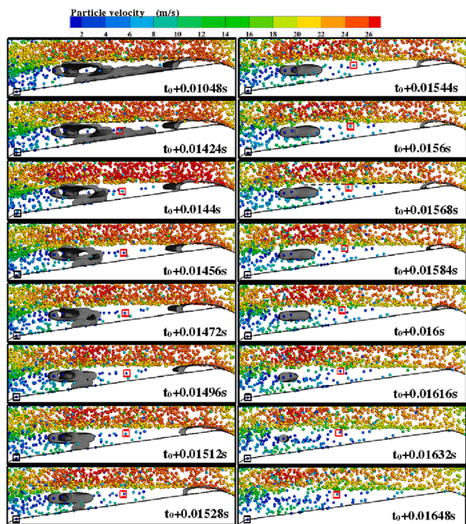
Fig. 28. Particle trajectory and cavity structure in Venturi tube [149].
