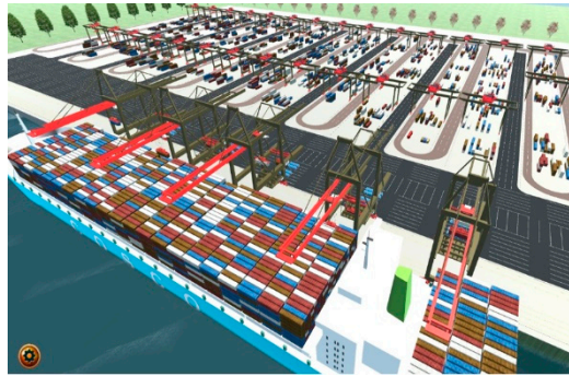
(a) Real-time monitoring interface of port crane
