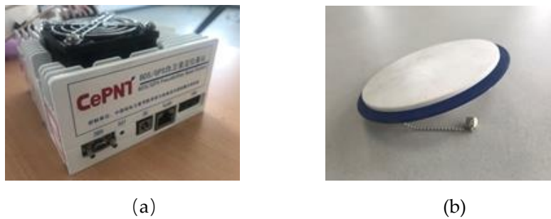
Figure 1. (a) pseudolite base station; (b) pseudolite antenna.
