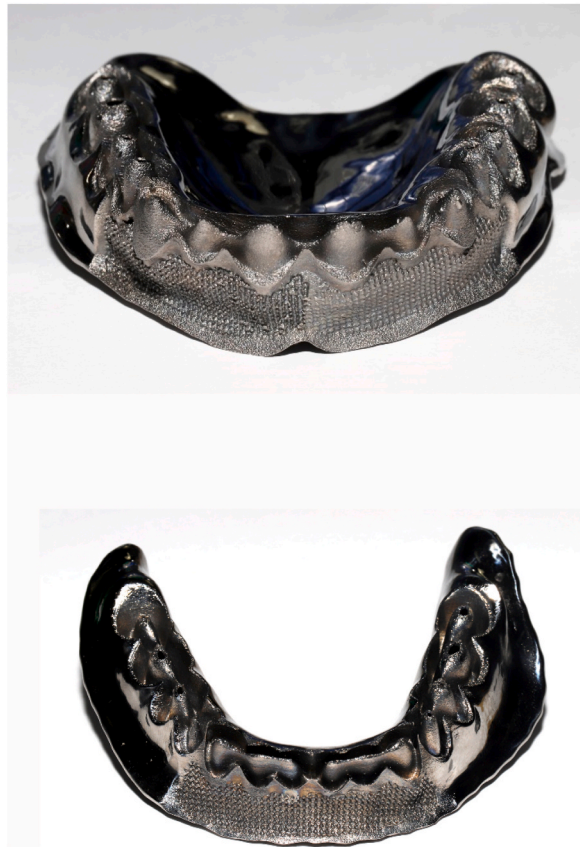
Fig. 5. Fabricate the titanium alloy base plates with abutment structures by the SLM method. A, Maxillary base plate. B, Mandibular base plate.
