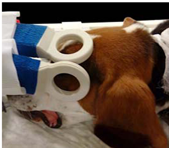
Fig. 1 Microcoil placement: the coils are placed at a 90° angle in relation to each-other, parallel to B0 (main static magnetic field), as close as possible to the orbit
