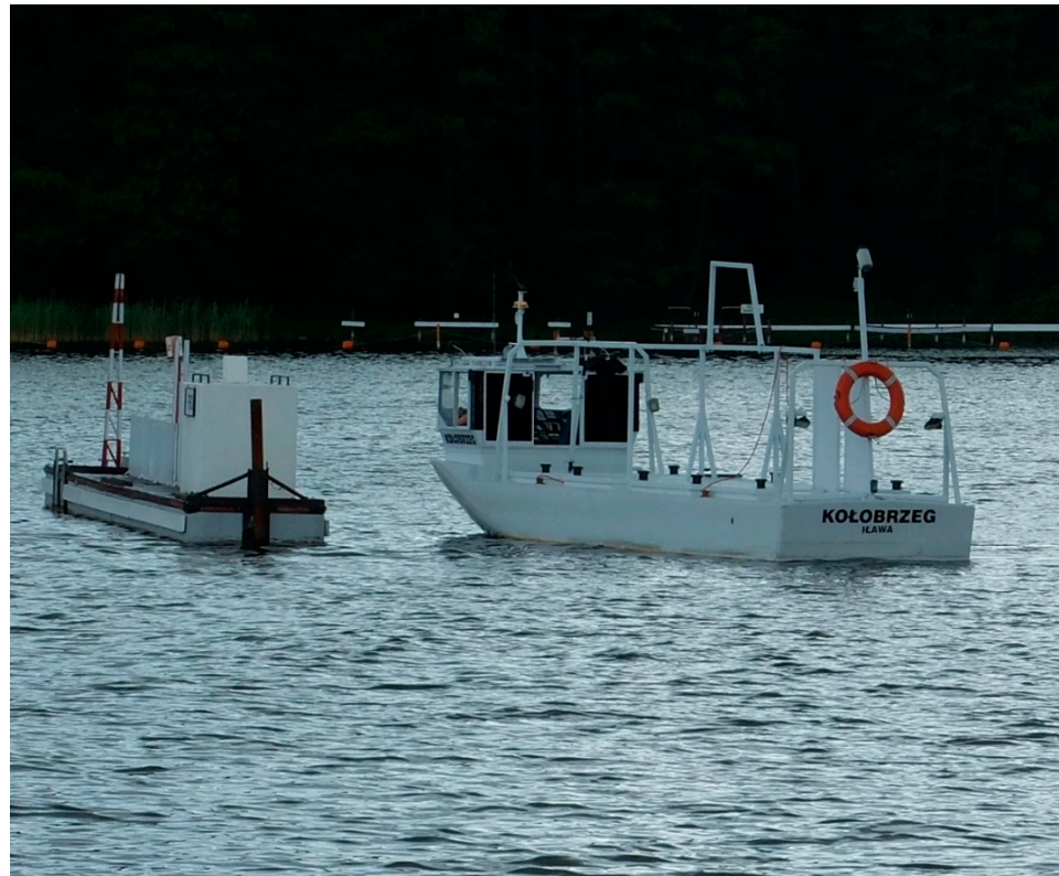
Figure 7. Physical model of the passenger ship Kołobrzeg used in the process of testing the AVAL technology.
