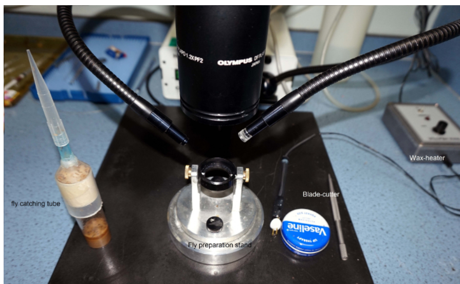
Figure 4. Tools and Devises Needed for Making the Fly Preparation. Fly catching tube is made by gluing a 1 ml plastic pipette tip to a 50 ml plastic centrifuge tube. Bespoke fly preparation stand enables free-rotation and locking of the fly-holder in a preferred position for preparing the fly. The fly is fixed by beeswax, using the electric wax-heater. Petroleum jelly is applied by a small applicator made by connecting a thick sort hair on a handle. Please click here to view a larger version of this figure.
