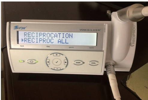
Figure 2 VDW Silver Reciproc endo-motor (Germany).
