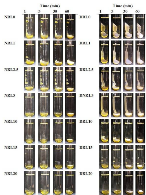
Figure 1. Gel formation of drug-free rosin-based in situ forming gel with various concentrations of LO using NMP and DMSO solvents in PBS pH 7.4 with different time intervals by visual observation. N = NMP, D = DMSO, R = rosin, L = lime peel oil.
