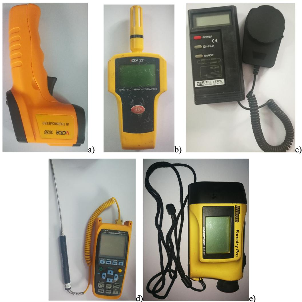
**Figure 2** The equipment used in this study. (A) Canopy temperature; (B) air temperature and relative humidity; (C) light intensity; (D) soil temperature; (E) tree height. Pictures by Wenjie Wang.
