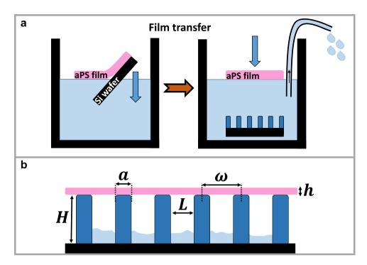
**Figure 9.** Schematic representation of the sample preparation. (a) Detaching the spin-coated polystyrene film from the substrate and transferring it on an array of pillars. (b) The film right after transferring (side view). Water may still be trapped in between the pillars.
