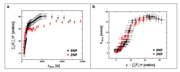
**Figure 4.** The dewetting velocity approached zero when elastic forces (visualized by the deformations of the pillars) acting at the contact line balanced capillary forces. (a) Mean tension,  $\sum_i |\vec{F}_i|/P$ , as a function of  $t_{\text{dew}}$ . (b)  $V_{\text{dew}}$  as a function of the sum of opposing capillary and elastic forces,  $\gamma_{\text{PS}} - \sum_i |\vec{F}_i|/P$ .
