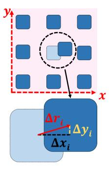
**Figure 1.** Pillars acting as force sensors. Sketch of the top view of the pillar array. One of the pillars has been deflected from its initial position. Knowing the modulus of the pillar and its size, the deflection  $\Delta \vec{r}_i$  can be translated into force components acting on pillar i in x- and y-direction.
