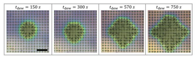
**Figure 7.** "Squaring the circle". Dewetting of a 400 nm thick film of polystyrene performed at  $T_{\rm dew} = 180$  °C on top of an array of deformable pillars for different values of  $t_{\rm dew}$ . The length of the black bar represents 50  $\mu$ m.
