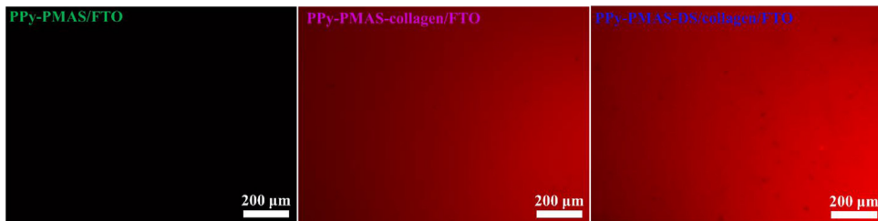
Fig. 3. Fluorescent labelling to identify successful collagen incorporation within PPy matrixes. Images of PPy-PMAS/FTO, PPy-PMAS-collagen/FTO and PPy-PMAS-DS-collagen/FTO after using the same fluorescent labelling method from our previous work [3]. Scale bar: 200 μm.
