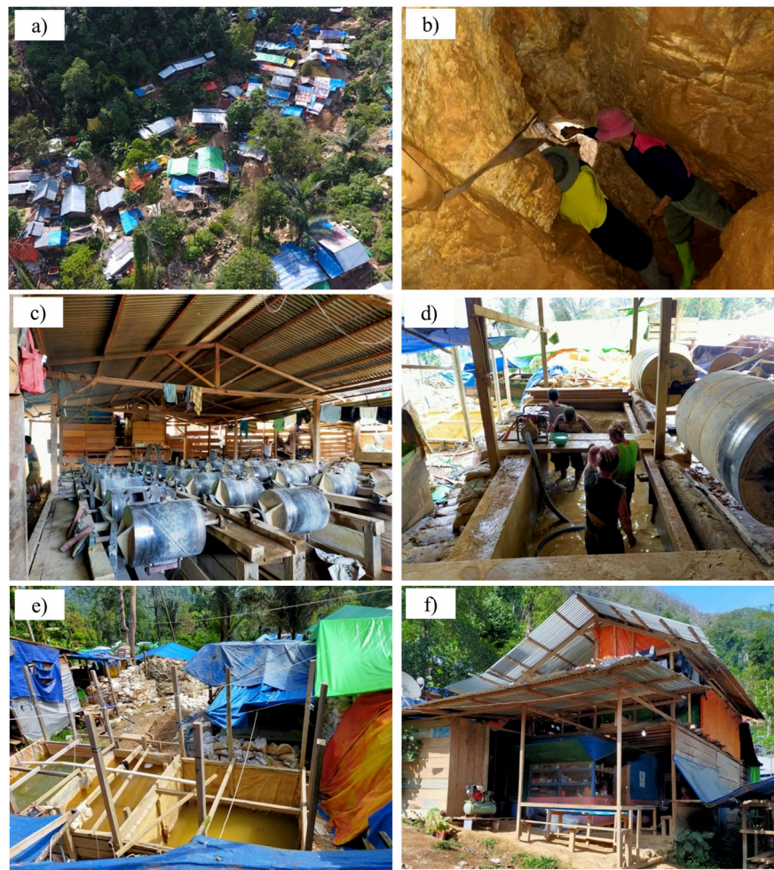
Figure 7. Motomboto ASGM camp. (a) Settlements in Motomboto ASGM 3 taken by an unmanned aerial vehicle. (b) An active mine hole. (c) Trommels for milling materials mined from holes. (d) A pool of water mixed with hydrogen peroxide for immersing the milled materials. (e) A pool of mercury mixed with cyanide for immersing the materials. (f) A common settlement where incoming miners and their families stay and manage a grocery shop.
