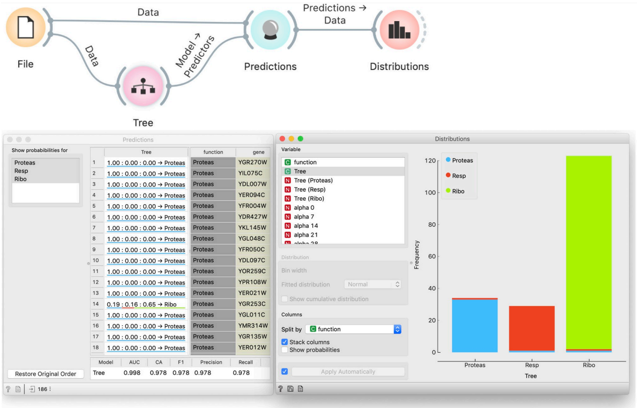
Fig 2. Incorrect evaluation of models. The tree is tested on the data from which it was induced. The Distribution widget shows perfect correspondence between the predicted and actual gene functions.
