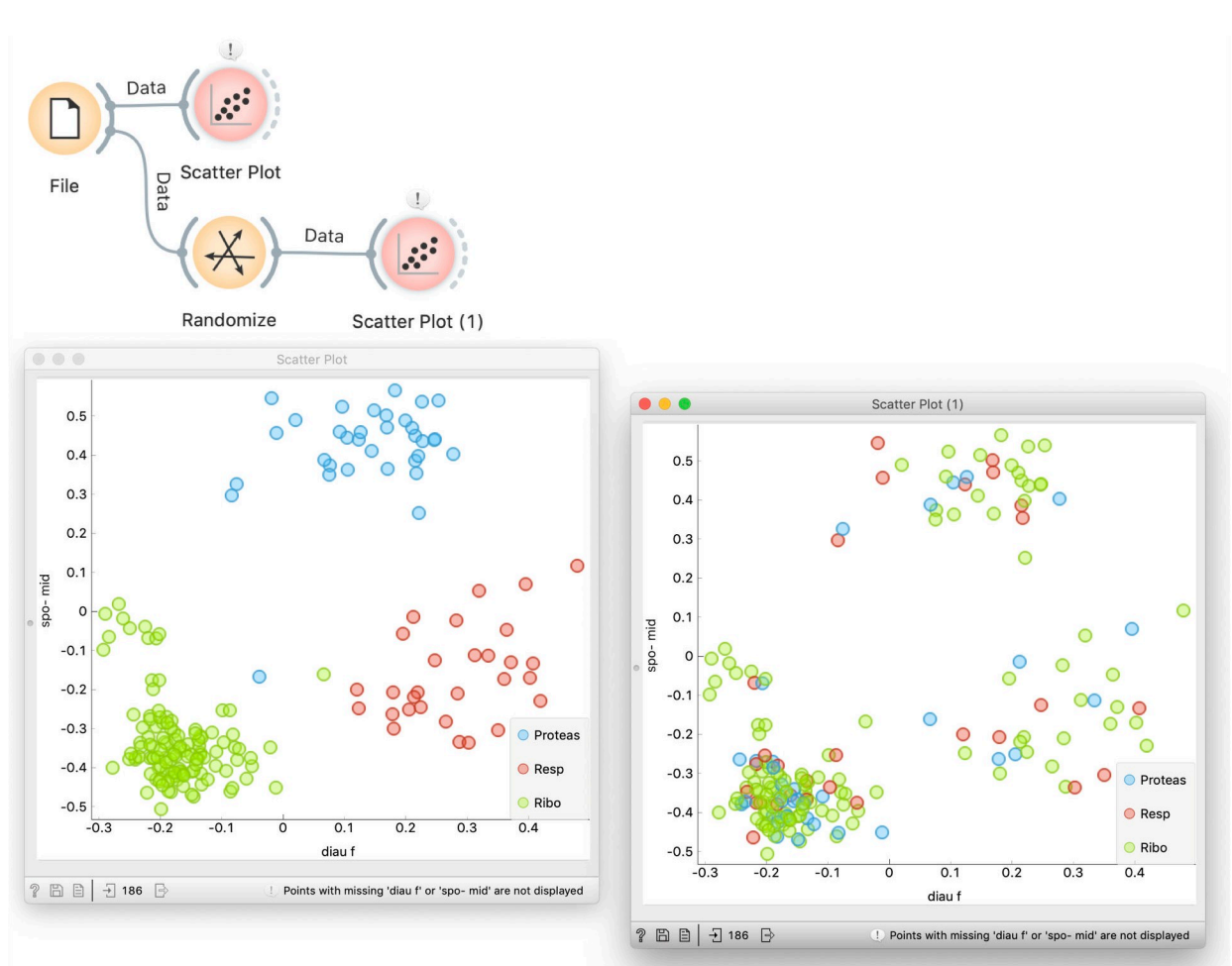
Fig 14. Exploring class-randomized data. Scatterplot in Orange can search for feature combinations that best split the classes. For the yeast expression data, diauxic shift ( diau f ) and sporulation at a five-hour timepoint ( spo-mid ) provide for the best combination. When the data is class-randomized, the class labels change, the pattern of class-separation is no longer there, but the data points keep their position. The effect of randomization is also visible by comparing the two Data Tables.
