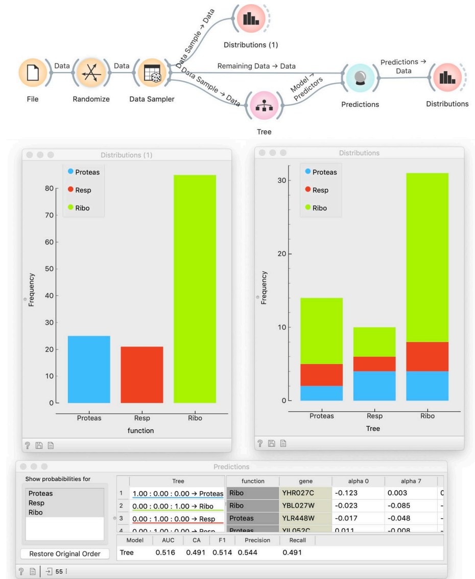
Fig 5. Testing a model on a separate data set. The Random Sample widget splits the data into two subsets, one for fitting and one for testing. Distribution of predictions by the model (right-hand histogram) roughly match the distribution of actual classes (left-hand side), but the actual class no longer matches the predicted.
