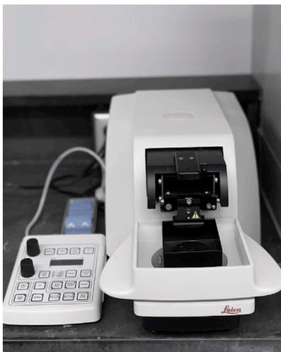
**Figure 2. Vibratome for sectioning brains**
