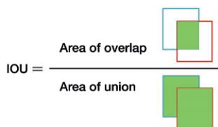
Figure 2. The formula with which the Intersection of the Union (IOU) was calculated.
