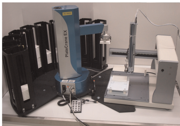
Figure 2. The robotic plate handler coupled to fraction collector.
