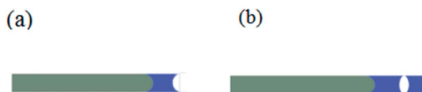
Fig. 2 Schematic diagram of slurry penetration process of spray coating method (a) first droplet of the slurry sprayed onto the end face of capillary tube; (b) subsequent slurry droplet sprayed onto the end face of capillary tube.
