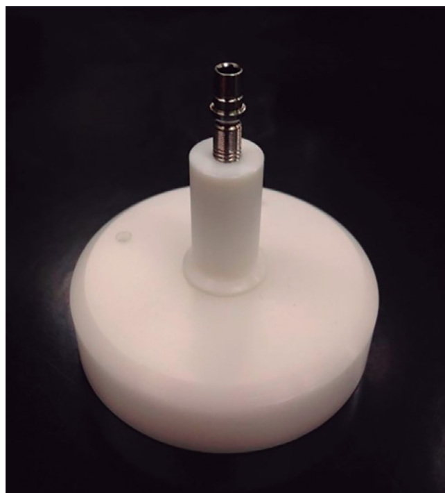
FIGURE 2 Teflon™ platform with implant mounted for micro-CT
