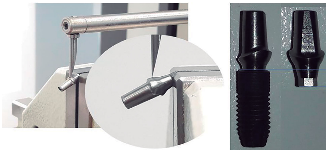
FIGURE 3 Profilometer, measurement of L dimension
