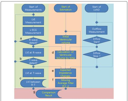
Figure 2 Algorithm for (left) detection of R-T impedance increases, (right) VAD operation conditions, and (middle and bottom) comparison of R-T impedance and prediction. (a) the R-wave detection in v-ECG, (b) the T-wave detection, (c) the calculation of LVI change during R-T period, (d) the prediction of volume change from v-ECG and LVAD inflow, (e) the impedance prediction, (f) the result of low-pass filter and (g) the comparison of the predicted value and the measured.
