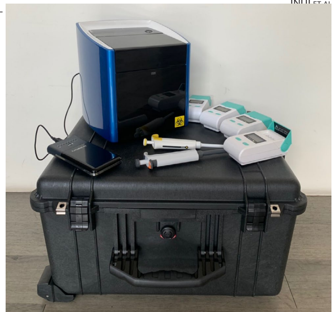
FIGURE 1 The iiRT-PCR portable setup. This Pockit Combo set includes a Taco mini portable extractor which runs on battery or net power, four Pockit mini DNA/RNA amplifiers, a set of pipettes, and a hard case suitcase for safe transportation to the field
