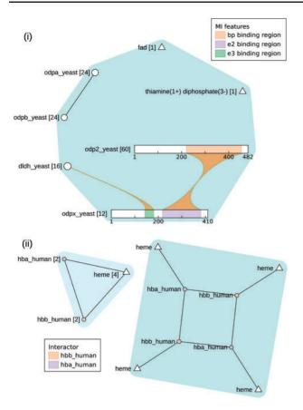
**Fig. 1.** (i) EBI-9691559: Mitochondrial pyruvate dehydrogenase complex. The complex (in blue) is a single n-ary interaction in which interactions between certain participants are known and some binding sites are known. Stoichiometry information is given in square brackets. (ii) EBI-9008420: Haemoglobin HbA complex. This complex is shown both with the stoichiometry information collapsed (left) and expanded (right)
