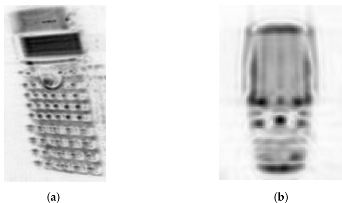
Figure 12. (a) Rotated SAR image of a calculator and (b) SAR image of the mobile phone in the frequency spectrum of 220–330 GHz.
